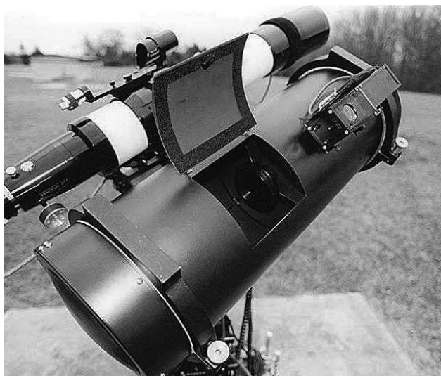
Fig. 5: Celestron's 8-inch f/1.5 Schmidt camera gave amateurs access to fast, sharp, wide-field astrophotography on Kodak's remarkable Tech-Pan film. Photo by Kent Kirkley.
