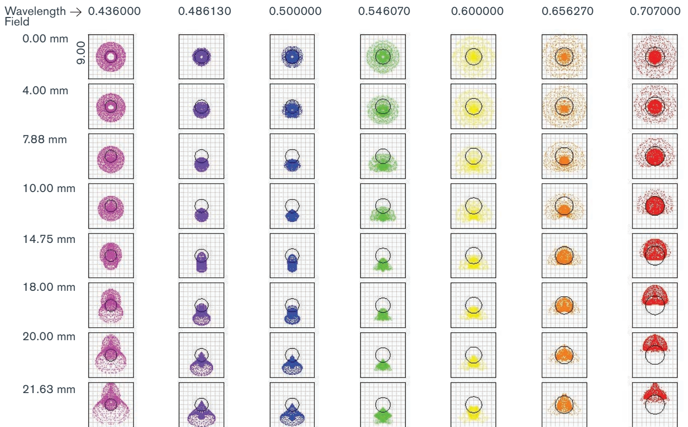
Fig. 10: The RASA's matrix spot diagram reveals that it forms remarkably tight star images across the entire visible spectrum from deep violet (0.43 \mu ) to near infrared (0.70 \mu ), from the center of the field to more than 21mm off axis. In practice, a field of view 52mm diameter is practical. The boxes are 9 microns on a side.
