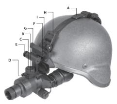
FIGURE 3-3. MOUNTING THE NYX-7 TO A HELMET
