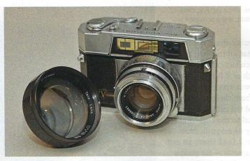
As mentioned in the text, the author used the Tele Lens accessory from his first 35-mm camera as a wide-field 1.8× astronomical monocular after being reminded of it by the first advertisements for the Omegon binocular. The lens and binocular are both based on a similar Galilean optical design.
