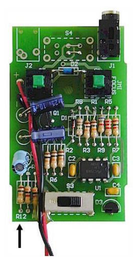
If the result is not what you expect, simply increase the resistance for a faster speed or decrease the resistance for a slower speed. Remember that this modification only affects the slow ("pre-ramp-up") speed. See the hand unit instructions for more information on speed and operation.
