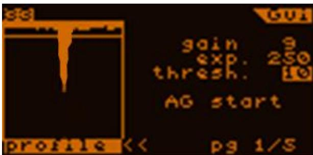
Fine focussing: In the guiding window (upper right corner shoes "Gui"), you can switch the live display between three modes entitled "Gui mask" (live view) "profile" (for focusing) and "drifts" (showing live the guide star movements you want to correct by guiding). Use the UP directional button to place the cursor onto the "<<" mark next to the name under the live view screen, and press SET to toggle between the modes. For focusing, we choose the "profile" screen.
