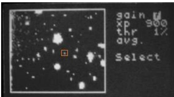
Using the live view, focus until stars appear smallest. Now mark "select" and press SET. A small rectangle appears on the screen, and you can use the directional buttons to move it and place it onto a star.
