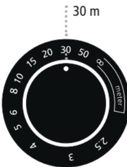
Using the distance scale on the dial of the central focussing wheel you can determine approximately the distance to the object in view.
