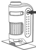
3. Adjust the zooming dial ④ to the desired level of magnification.
