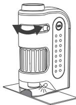
4. Rotate the focusing ring ⑥ until the image is sharp and clear.
