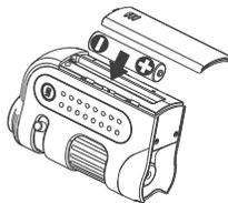
3. Attach the battery door ① as shown below.
