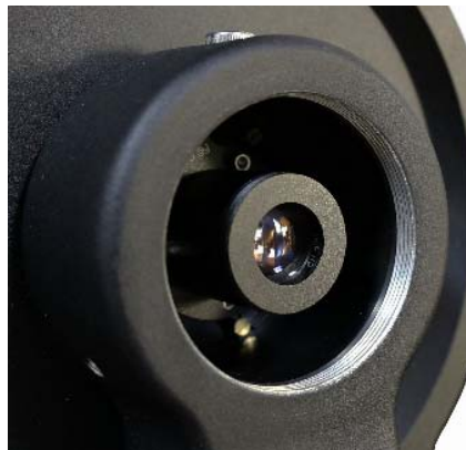
Figure 17. CEM120 with an installed electronic polar scope
