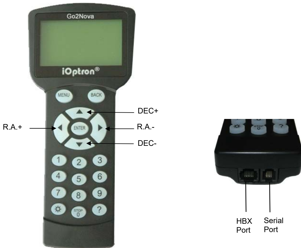
Figure 8. Go2Nova ® 8407+ hand controller
