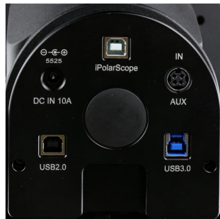
Figure 7. Cable Management System Input Panel
