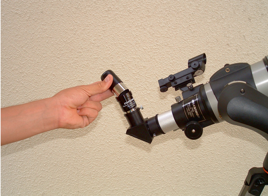
Fig. 2.21 Inserting an eyepiece into a Barlow mounted in a diagonal (Photo courtesy Tommy McGee)
