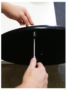
7. Now gently tighten the assembly until it is just snug by turning the screw (h) with the included 3/32 Hex Wrench (k) while holding the 8-32 Nylon Insert Lock Nut (j) still. You will find that there is no easy way to get a socket in there or otherwise hold the lock nut while turning the screw. But this is a good thing because it will prevent you from overtightening the screw and
