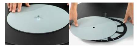
3. Leave the threaded center insert in place (it came already firmly fixed in the center hole of the ground board when purchased). Remove the two plates and the "wagon wheel" (with needle bearings) from the ground board. Set aside (they won't be needed). Also set aside the Axle Sleeve (the plain tube resting on top of the center insert). The Axle Sleeve won't be needed.
