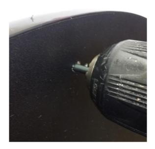
5. IMPORTANT: Drill out the holes that the foot screws were in with a 5/32" drill bit. If you skip this step, you will ruin the Teflon when you re-install and tighten the feet.
