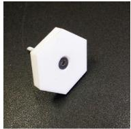
Now insert the screws with the Teflon Foot Bearings into the foot holes that you drilled out earlier. Note that you are going to **BOLT** the Teflon Foot Bearings onto the ground board. The screw (h) should slip though the ground board without you having to screw it in. (This is why you drilled out the hole earlier using your 5/32" drill bit).
