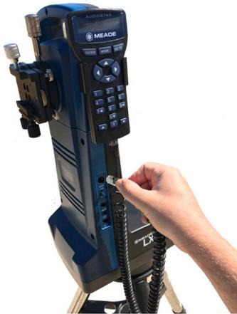
**8** Be sure the telescope power switch is in the off position. Remove the handbox and the coiled interface cable from the packing materials. Plug one end into the HBX port of the control panel and plug the other end into the Handbox port on the LX65 handbox.
