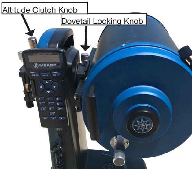
**9** Loosen the Dovetail Locking Knob slightly. Carefully place the telescope optical tube's dovetail into the dovetail saddle on the LX65's fork mount, then tighten the Dovetail Locking Knob. When standing behind the LX65 facing the control panel, the optical tube should be on the right hand side of the fork mount.
