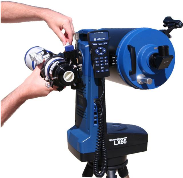
The LX65 is equipped with a second dovetail saddle to allow attachment of a second optical tube assembly. The optical tube must have a Vixen-style dovetail plate to attach to the LX65. The practical weight limit for the second optical tube is 7 lbs.
