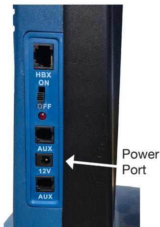
**7** Use only the optional Meade Universal AC Power Adapter (part number 07584) with your LX65 telescope when connecting to AC power. Power adapters from other manufacturers may cause damage and void your warranty.
