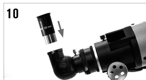
Insert the barrel of the 25 mm eyepiece into the diagonal and tighten the set screw.
