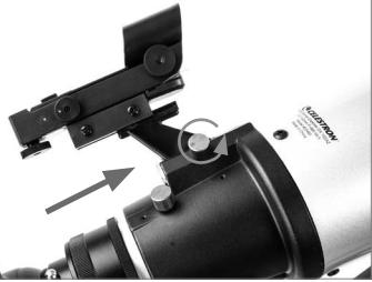
Slide the finderscope bracket into the dovetail slot on the telescope tube near the focuser. The large window on the finder should be facing the front of the telescope. Secure the bracket by tightening the setscrew on the dovetail slot.
