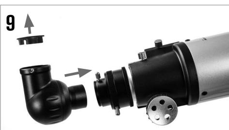
Locate the erect image diagonal and remove the plastic covers. Insert the barrel of the diagonal into the focuser and secure in place by tightening the set screws.
