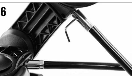
Place the slow-motion control knob over the D-shaped gear shaft and push inward to make sure it is fully seated. Use the hex key to tighten the setscrews onto the gear shaft. Return the hex key to its storage position in the front of the mount.
