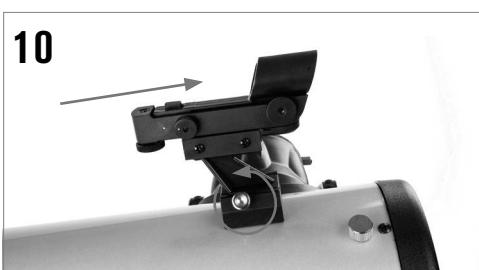
Slide the finderscope bracket into the dovetail slot on the telescope tube near the focuser. The large window on the finder should be facing the front of the telescope. Secure the bracket by tightening the setscrew on the dovetail slot.
