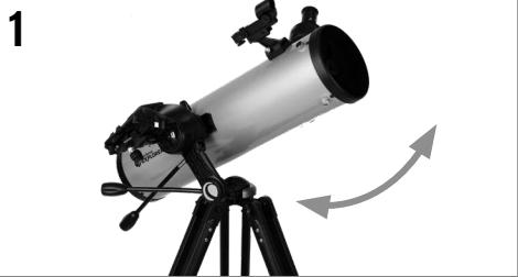
The StarSense Explorer DX mount has slip clutches in both axes. To make large movements with the telescope, simply hold a tripod leg with one hand and use the other hand on the telescope tube to push the telescope in the desired direction.
