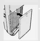
6 put filter 1 back the machine. Make sure the side with plastic pull faces towards you.
