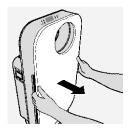
Use clean water or dust collector to get rid of dusts remains on the pre-filter. Please make sure the pre-filter is dry before putting it back into the machine.
