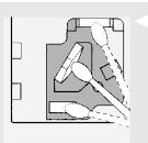
3 use wet cotton swab to clean the sensor the air intake and air outlet.
