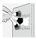
Caution: when air humidity inside the room is high, there may be condensate water remaining on the sensor. In this case, the sensor may not be able to detect the air quality. Accurately. Please clean the sensor to make sure the machine works in good condition.
